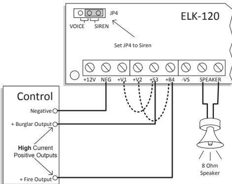
Set JP4 to Siren. All current must be supplied from the Burg and Fire Outputs on the Control. Average current draw with 8 Ohm speaker load is 1.2 Amps, or 1.8 Amps with 4 Ohm load.
