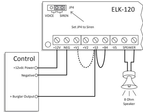
Set JP4 to Siren. Industrial horn will play if +S3 and +B4 are connected and activated together. Adding a wire jumper between +S3 and +V1 will combine the Horn with Voice 1 Channel.
