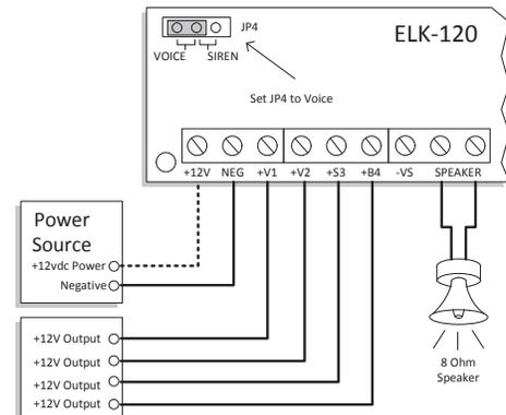
Set JP4 to Voice. A recordable voice channel may be played by connecting 12 Volts DC between the NEG terminal and the positive (+) channel input. For low current triggering of a channel, or to have messages play through to the end when activated by a momentary trigger, connect terminal +12V to a constant +12 Volt DC source.
