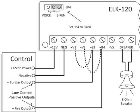
Set JP4 to Siren. The operating current is drawn from the constant +12 Volts DC power source. The +V1 and +B3 channel trigger terminals draw only 30 mA each from the control alarm outputs.
