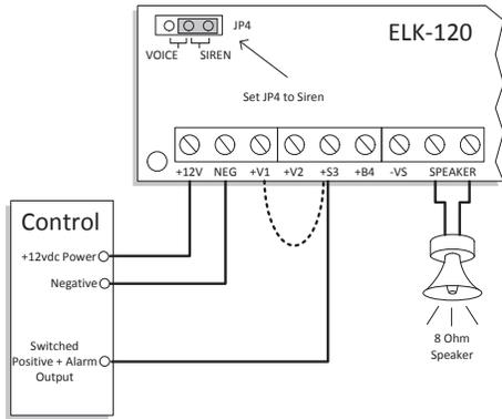
Set JP4 to Siren. A Steady +12 Volts DC applied to +S3 activates the Siren sound. A 1/2 to 1.5 second Pulse to +S3 activates the Horn sound. Adding a wire jumper between +S3 and +V1 will combine the Siren sound with Voice 1 Channel, or Pulsing +S3 combines the Horn sound with Voice 2 Channel.
