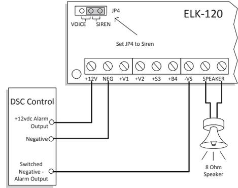
Set JP4 to Siren. This method is great for Controls that switch their negative alarm output (eg: DSC). A Steady Negative to terminal -VS plays the Siren sound combined with Voice 1 Channel. A 1/2 to 1.5 Second Pulse to terminal -VS plays the Horn sound combined with Voice 2 Channel.
